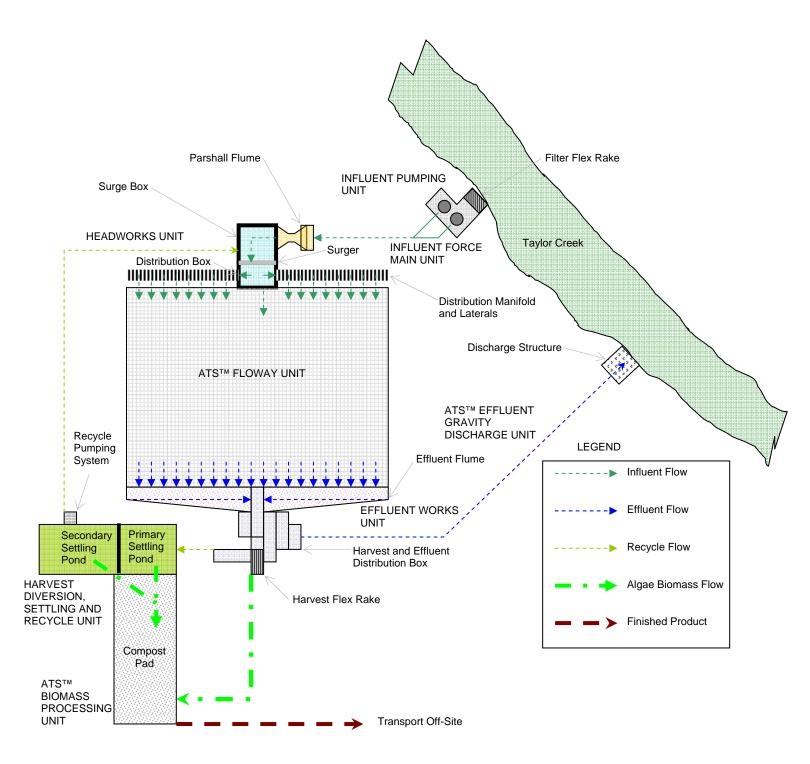
Figure 2.1-1 Process Flow Schematic (NTS)
